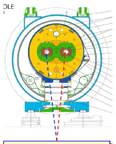
LHC: Identical bending field in both apertures of two-in-one dipole
